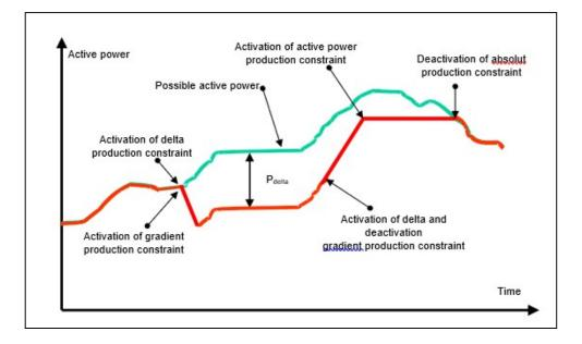
Figure 14: Active power control functions for a Renewable Power Plant
