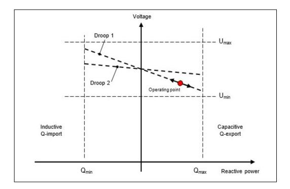
Figure 13: Voltage control for the RPP
