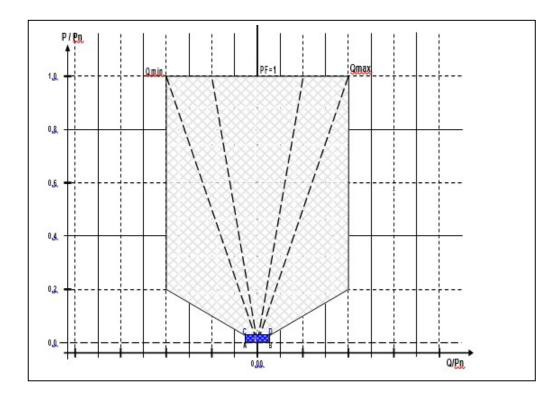
Figure 10a: Reactive power requirements for RPPs of category C at the POC (Qmin and Qmax are voltage dependent as defined by Figure 11)
