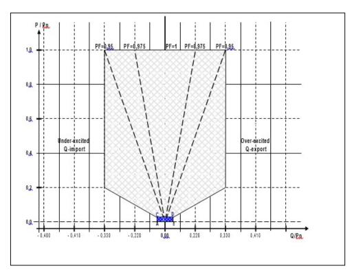
Figure 10b: Reactive power requirements for RPPs of category C (at nominal voltage at POC)
