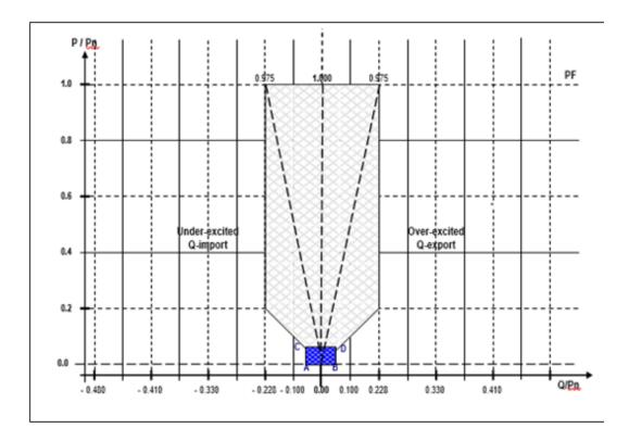
Figure 8a: Reactive power requirements for *RPPs* of *category B* at the *POC* (Qmin and Qmax are voltage dependent as defined by Figure 9)
