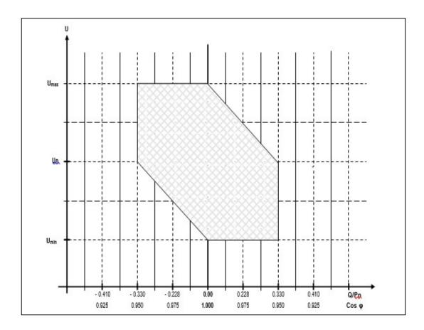
Figure 11: Requirements for reactive power and voltage control range for RPPs of category C
