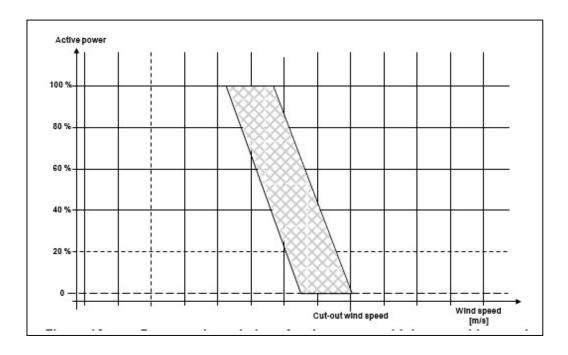
Figure 16: Downward regulation of active power at high renewable speed
